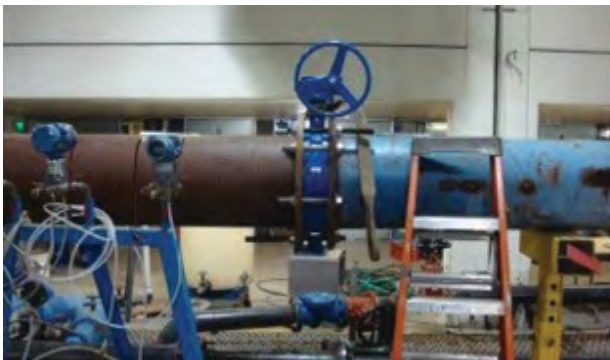
BF SERIES WAFER / LUG BUTTERFLY VALVES BEING TESTED AT AN INDEPENDENT RESEARCH LABORATORY
