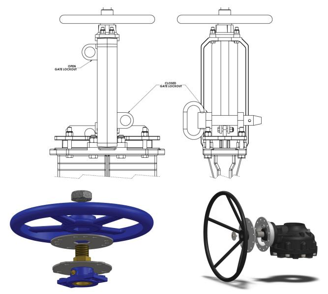
Gate lockout packages are available as open or closed only, or both open and closed. Lockout packages come in 3 types:
