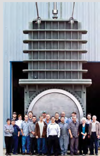
Left: 96" Figure 193 bonneted knife gate valve, 65 PSI CWP, one integral seat with EPDM seal and one replaceable seat ring with EPDM seal to provide tight shut off in reverse flow. Full pressure rated bonnet and Rotork electric motor. Three were built for use in a water treatment plant.
